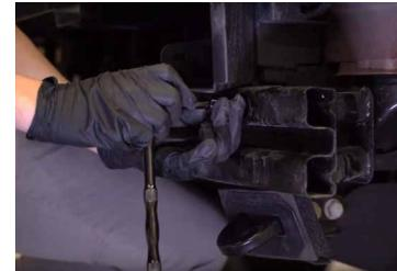
9. Reinstall the crash bar using the original 15mm bolts. Secure the bolts to 43 foot pounds.
