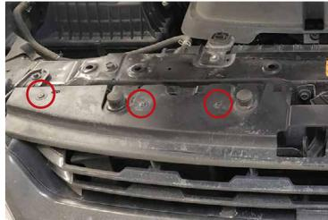
3. Remove the six T15 torx screws holding the top of the grille to the radiator core support.
