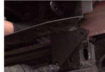
8. Maneuver the light bar brackets through the air duct and set them in place in the same orientation as the image above.
