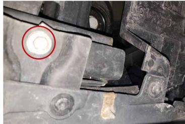
4. From underneath the truck, remove the two 10mm hex bolts securing the bumper to the frame of the truck.
