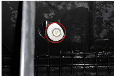
5. Remove the two 10mm bolts inside of the lower grille securing the bumper to the frame.
