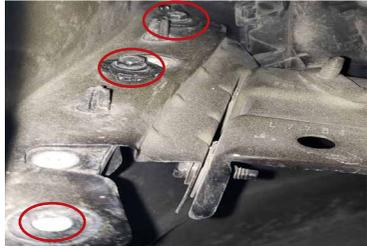
2. Remove the three 7mm bolts inside of the fender to detach the bumper from the fender. Then disconnect the fog light harness.
