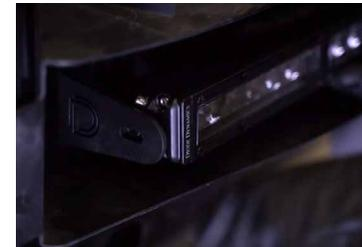
10. Install your new 30" light bar on the brackets using the included 10mm bolts on either end. We recommend hand-tightening these bulbs initially to allow you to aim the light bar later.
