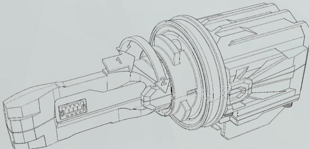
The proper alignment of the 2Stroke 3.0 bulb's LEDs is left and right, horizontally, as shown below. This alignment ensures the optical efficiency of the lamp assembly is fully retained.
