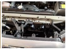
Step 4: Remove the two remaining white clips holding fog light shrouds to bumper.
