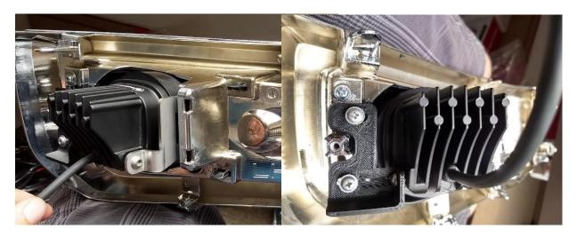
Step 8: Install shrouds with Squadrons onto vehicle the reverse of removal.
