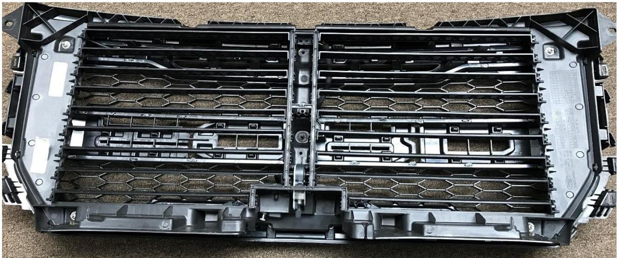
7. Separate the two sections of the grille and lay the inner-grille down, with the front facing upward.
