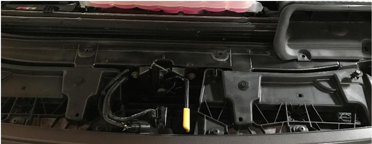
3. Gently pull on the painted fascia piece around headlight starting with the upper most section, closest to the push pin that was removed in the previous step. You will hear a distinct “pop” when the shroud is disconnected.
