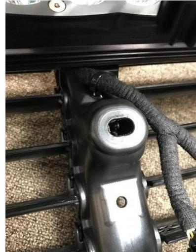
**NOTE: Make sure wiring is routed down the correct side, as shown in the picture above.**
