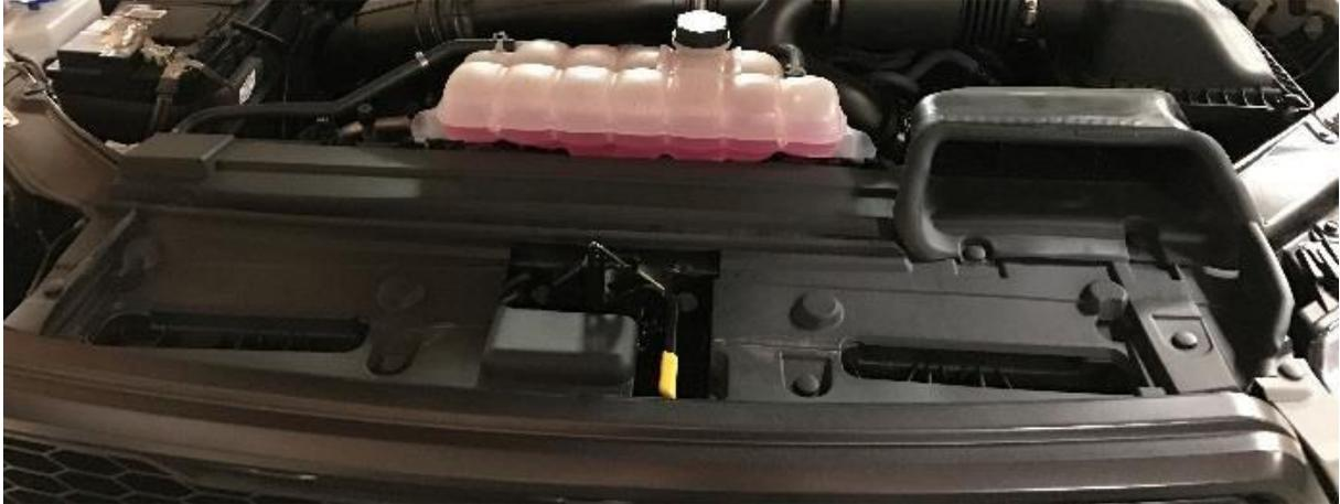
2. Disconnect the two wiring connectors, and the quick-disconnect for the fluid washer fluid hose. Then remove the four bolts securing the front grille, shown below.
