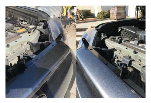
6. Now it is time to mount each light into a bracket. Using a 7/16" socket, tighten the provided ¼" diameter bolt with washer through the bracket into the light housing. Make sure that the desired angle is set at this moment. The entire light/bracket assembly will have to be removed to make adjustments. Place the 5/16" bolts and accompanying washers through the bracket.
