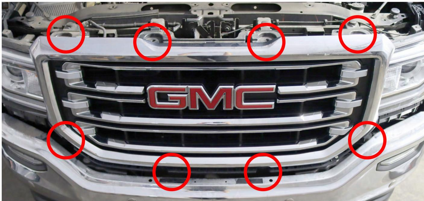
Take out the 10mm bolt from the bottom corner of the grille, one on each side.
