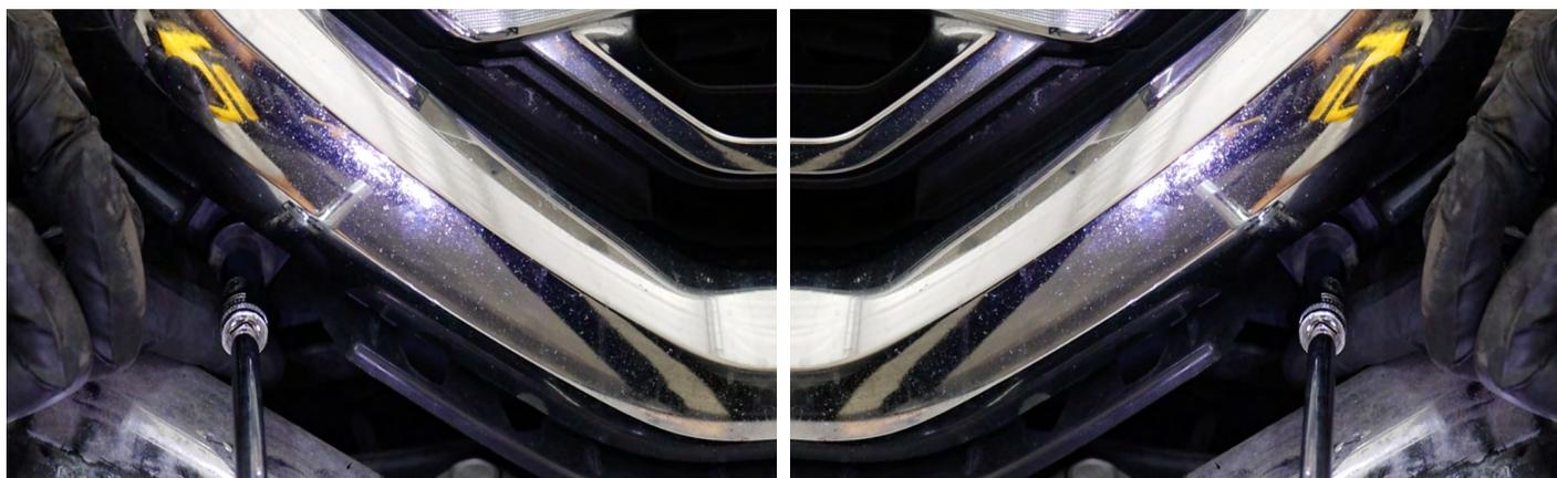
Unscrew and remove the two 10mm bolts from the center bottom of the grille.
