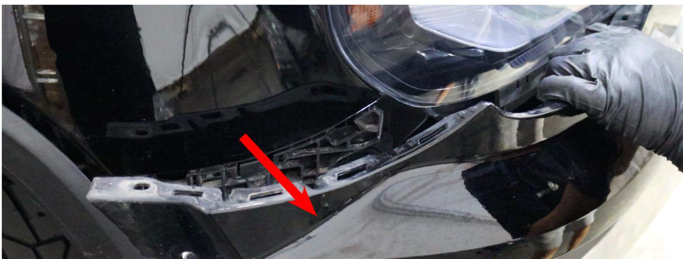
Once both ends of the trim piece are partially removed, use a panel popper to work at the middle. Carefully remove the trim piece by releasing it from all of the clipping points.
