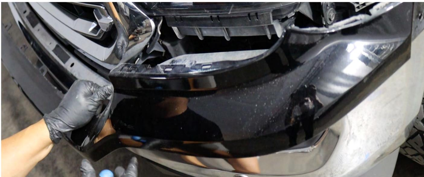
Once the trim piece is removed, set it aside for later reinstallation.
