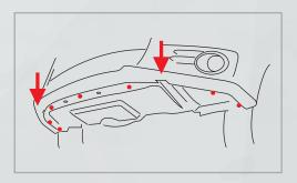
Remove the sidemarker by inserting a slotted screwdriver to release the clip inside the sidemarker housing.
