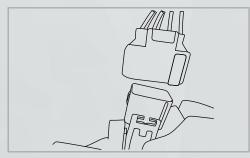
Factory Halogen Cars: Connect the provided 8-pin to 6-pin adapter harness between the XB LED lamp and the factory connection.
