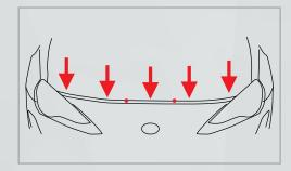
With the sidemarker removed, remove the plastic push-rivets.
