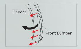
Remove the screws (red arrows) and plastic pop rivets (circled) centered on the bottom of the front bumper.
