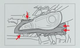
Remove the screws (red arrows) on the OEM headlights. The headlight can now be removed from the vehicle.
