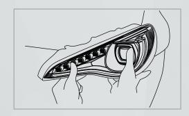
Disconnect the OEM leveling motor connector. (if applicable)
