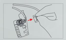
Factory HID Cars: Connect the OEM connector to the XB LED headlight connection directly.
