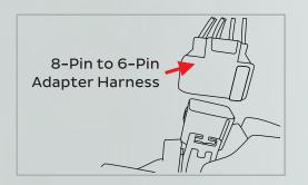
2017+ US Cars: Connect the adapter harness with headlights. Then, connect the vehicle plug to the adapter harness. Finally, remove the installed harness.
